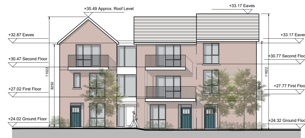
DUPLEX BLOCK C EAST ELEVATION (STREET ELEVATION)
